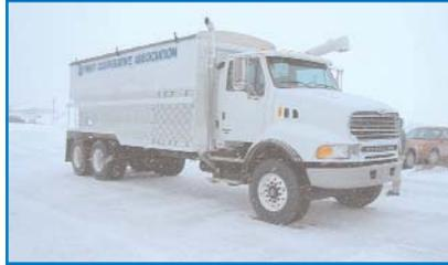
*A new bulk feed delivery truck has been added to our Feed Team fleet to help us provide timely, efficient delivery of rations to the livestock producers and operations we serve. The new truck has one 4-ton and three 3-ton compartments, and when enables us to bring 13 tons of feed out with every trip to the country.*
