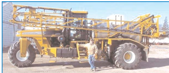
Our 2007 TerraGator 6203 Is VRT-Ready For Service It's shaping up to be a busy spraying season all across FCA Country this spring, and the addition of the new 6203 TerraGator gives us the capability to spray liquid nitrogen using Variable Rate Technology to bring added efficiencies to your fields.
